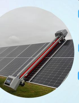
Ultra-soft PBT bristles with water resistance properties enabling all weather operation
